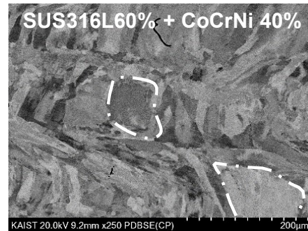
[ SUS316L → CoCrNi SEM Analysis (x250) ]
